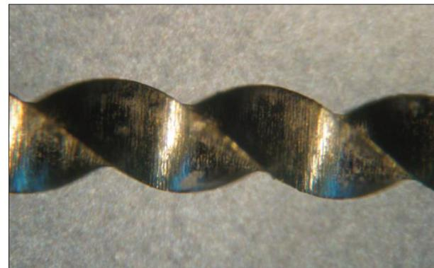
**Figure 6.** Residual film of calcium hydroxide on a size 35 file treated in an ultrasonic bath with disinfectant solution
