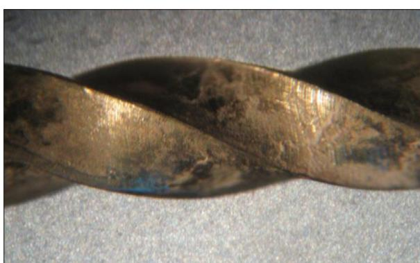
**Figure 5.** A size 25 file with residual deposit of calcium hydroxide over the entire surface (score 2)
